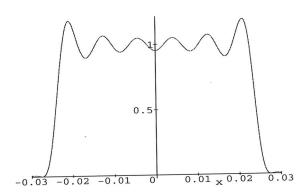
Notice that the intensity modulation of the image (fringes) is due to coherent illumination of the object and finite size of the square pupil (diffraction limited imaging).
