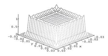
If the sides of the pupil are halved then the function h is changed. We calculate the resulting image intensity below, where a trailing s is used to denote the results with the smaller aperture.
