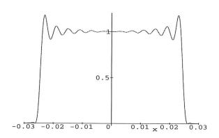
The above calculations were restricted to the one dimensional case. For this optical system (and for many others) the functions are separable and thus Ii(x, y) = Ii(x)Ii(y). A plot of Ii(x, y) is shown below.
