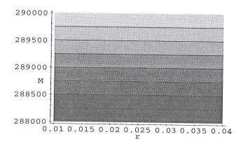
The change in the surface with respect to r is extremely small compared to that with respect to M. It's quite difficult to find a minimum on so uniform a surface. This problem is similar to "stiffness" encountered in differential equations.
