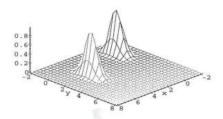
The gaussian peak in the background is the original function. The peak in the foreground shows the shift of 5 units in the x direction and two units in the y direction.
