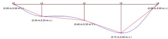
Figure 2: trapezoidal rule. measured data point:  $(x, d, v)$
