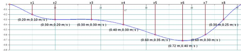
Figure 1: cross section of a river. measured data point:  $(x, d, v)$
