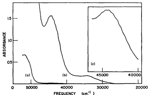
FIG. 1. Electronic absorption of methanal- $\text{h}_2$  azine. Gas pressure is 15.0 torr, path length in (a) 1 mm, (b) and (c) 100 mm. 1(c) is expanded portion to illustrate diffuse structure of second band.
