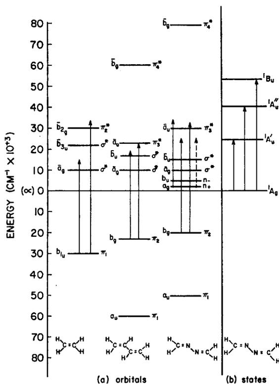
FIG. 3. Approximate energy levels of (a) orbitals of ethene, butadiene-1,3, and methanal azine, and (b) singlet states of methanal azine. Energy levels from simple Hückel calculations have been scaled to suit assigned transitions.
