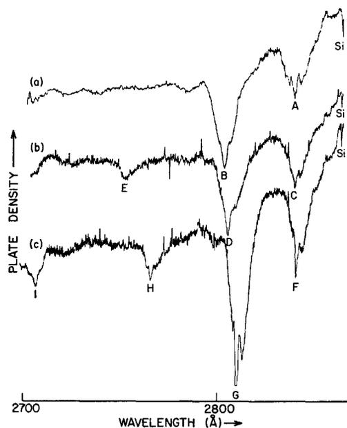
FIG. 2. Microdensitometer traces of transient absorption spectra photographed after flash photolysis of (a) methanal- $h_2$ , (b) methanal- $hd$ , and (c) methanal- $d_2$  azines. Scans have been displaced vertically. Source absorption line at right is SiI, 2882 Å; wavelength scale is nonlinear.
