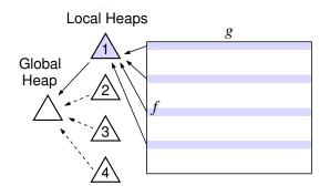
One heap per core. Add (merge) results in global heap.
