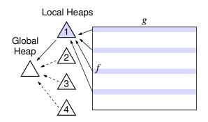
One heap per core. Add (merge) results in global heap.
