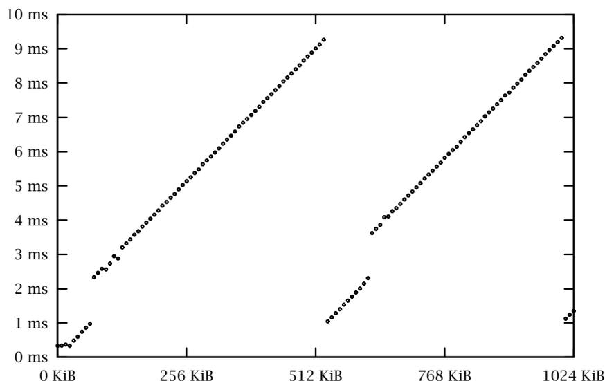
**Figure 1:** Access times versus file offset. From offset 528 KiB to 536 KiB there was a drop of 8.2 ms, which tells us that this was made on a 7200 RPM disk.
