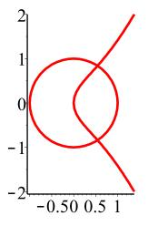
You can read off from the plot roughly where the curves intersect. Using the **fsolve** command compute the \_intersection points accurately.
